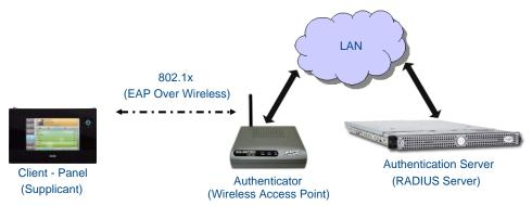
FIG. 93 EAP security method in process
